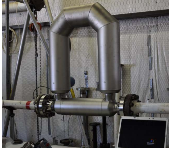
A Coriolis Flowmeter being Calibrated at CEESI Photo by Flow Research
